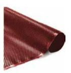
Powerful drainage membranes made of polyethylene with dimples. The thickness of the membrane is 0,5 mm and the density is 500g/
