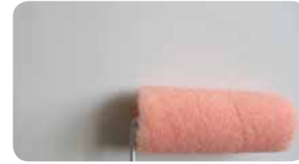
STEP 7: Apply GLX 292 FLEX PRIM , deep penetration primer.
